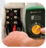
If you have some hot water, but not as much as you're used to, use a voltmeter and check the incoming voltage. See the wiring diagram and the water heater's label for power (voltage) requirements. Also, check the temperature setting on both thermostats—see Step 6.
