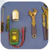
You'll need common plumbing tools and pipe joint compound (or Teflon® tape) approved for potable water. You'll also need a circuit tester or voltmeter. Most codes require the water heater to be installed in a metal drain pan. See the Installation Instructions for information about sizing the drain pan and other installation details.
