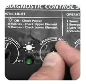
Check your work using the wiring diagram and the printed instructions. Reinstall the plastic cover and screws. Set the Temperature Control to 120 degrees. *Set the Mode Control to Energy Smart Mode.*
