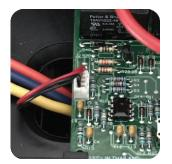
Install the Temperature Sensor Plug. The Plug is made to fit only one way, and will insert easily if properly aligned.
