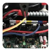
Using pliers, remove the yellow, orange and blue wires, pulling gently on each terminal.
