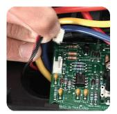
Pull the Temperature Sensor Plug up and away from the Control Board.
