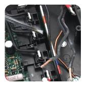
Push on the locking tab with a flat-blade screwdriver to release the Control Board.
