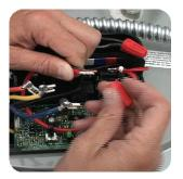
Disconnect the black and red power supply wires.
