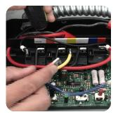
Inspect the yellow, red and blue wires for damage. If the wires are damaged, use the replacement wires that came with the kit. *Reconnect the wires using the color code on the box as a guide.* Each wire terminal must be FULLY inserted and must fit tightly. Replace a terminal if it is loose. Loose terminals can overheat and damage the Control Board.
