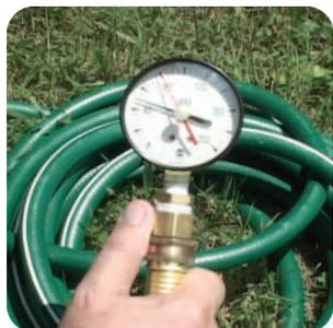
To install a Thermal Expansion Tank, first determine the water pressure in your home. Use a pressure gauge with a recording hand, and check the pressure for a 24-hour period.
