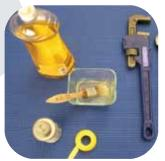
You'll need common plumbing tools and pipe joint compound (or Teflon® tape) approved for fuel gas. You'll also need leak detection solution. You can use children's soap bubbles or hand dishwashing soap mixed with water. Most codes require the water heater to be installed in a metal drain pan. See the Installation Instructions for information about sizing the drain pan and other installation details.
