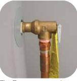
The Temperature and Pressure Relief Valve (T&P) is an important safety device. It opens to relieve pressure if the water temperature or pressure is too high. Use the new one that came with your new water heater. Don't reuse the old T&P valve.
