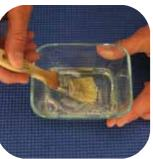
To check for gas leaks, use children's soap bubbles or hand dishwashing soap (mix one part soap to 15 parts water) or a commercial gas leak detection solution. Do not use an open flame to check for gas leaks!
