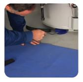
Use a household brush with plastic bristles to clean the Flame Arrestor. Clean using an in and out motion.
