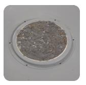
*Pilot outages can sometimes be caused by a dirty Flame Arrestor or Filter Screen, and that dirt could be blocking air needed for combustion.* Usually the Flame Arrestor or Filter Screen is blocked with dust or lint and can be cleaned with a common household brush and a vacuum cleaner.
