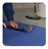
Vacuum any lint from the brush and repeat brushing and vacuuming until the **brush is completely clean**.
