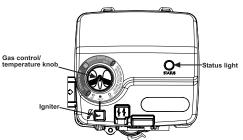
IMPORTANT: If the pilot will not stay lit after several tries, turn gas control/temperature knob to "OFF" and check the status light for flash codes. Record any codes and call your service technician or gas supplier.
