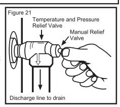
drain. Standing clear of the outlet (discharged water may be hot), slowly lift and release the lever handle on the temperature and pressure relief valve to allow the valve to operate freely and return to its closed position. If the valve fails to completely reset and continues to release water, immediately shut off the manual gas control valve and the cold water inlet valve and call a qualified person.
