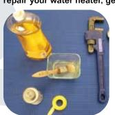
You'll need common plumbing tools and pipe joint compound (or Teflon® tape) approved for fuel gas. You'll also need leak detection solution. You can use children's soap bubbles or hand dishwashing soap mixed with water. Most codes require the water heater to be installed in a metal drain pan. See the Installation Instructions for information about sizing the drain pan and other installation
