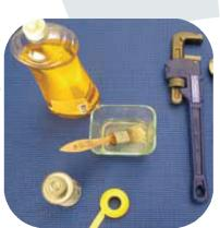
You'll need common plumbing tools and pipe joint compound (or Teflon® tape) approved for fuel gas. You'll also need leak detection solution. You can use children's soap bubbles or hand dishwashing soap mixed with water. Most codes require the water heater to be installed in a metal drain pan. See the Installation Instructions for information about sizing the drain pan and other installation details.
