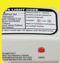
The Status Light will blink once every three seconds when the Pilot is lit and the unit is working normally. If the Status Light does not begin to blink after 90 seconds, STOP. Turn the gas control knob off. Wait 10 minutes before attempting to relight the unit. It may take 2-3 attempts to light the Pilot on a new water heater. If the Status Light turns solid red when you release the control knob, turn the control knob off and wait 10 minutes before relighting the Pilot.
