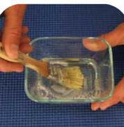
To check for gas leaks, use children's soap bubbles or hand dishwashing soap (mix one part soap to 15 parts water) or a commercial gas leak detection solution. Do not use an open flame to check for gas leaks!
