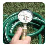
To install a Thermal Expansion Tank, first determine the water pressure in your home. Use a pressure gauge with a recording hand, and check the pressure for a 24-hour period.
