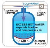
Thermal Expansion Tanks contain an air bladder which is pressurized with air, and expands and contracts to absorb the expanded water from the water heater.
