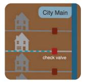
In the past, this extra gallon or two made it's way back in to the city's water supply every time the water heater ran. But changes in plumbing regulations required that Backflow Preventers, or Check Valves be added to homes to keep the water in your home from possibly contaminating the public water supply.
