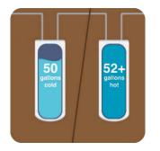
Water expands when heated. A 50 gallon tank of cold water becomes about 52 gallons or more when the water is hot.
