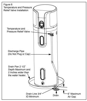
For protection against excessive pressures and temperatures, a temperature and pressure relief valve must be installed in the opening marked "T & P RELIEF VALVE" (See Figure 5).
