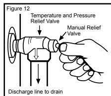
pressure relief valve to allow the valve to operate freely and return to its closed position. If the valve fails to completely reset and continues to release water, immediately disconnect the electrical power, close the cold water inlet valve and call a qualified person.
